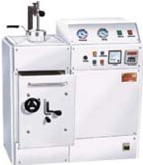
Gambar 7. Vacuum Casting Induction Furnace.[2]
