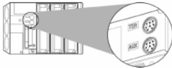
Figure 3. Terminal Port on TSX Micro 37-21 PLC
