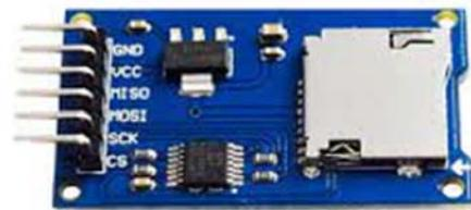
Gambar 8. Modul Micro SD Card
