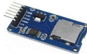
Gambar 5. Modul Micro SD Card
