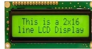
Gambar 4. LCD 2x16
