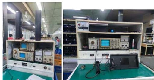
Gambar 1. Quality Control PCB Power Amplifier Secara Manual
